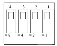
If you are installing a parlour up to 16-a-side the left side relay card would be addressed "1" and the right side relay card would be addressed "2".
