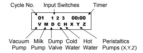
To the right of the cycle number, the numbers 1, 2 and 3 are displayed. These represent the settings for the three switch inputs I/P1, I/P2 and I/P3. The space to the left of the number indicates the current condition. If the space to the left of number 1 is a blank space the switch is not selected. If the space to the left of number 1 is a *right pointing arrow* the switch is selected.
