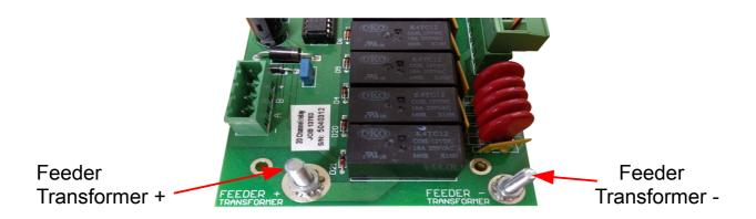
Normally with a 12 volt D.C. system the negative connections on all the feeders are linked together and directly connected to the feeder transformer.
